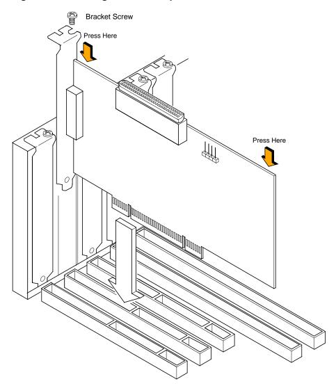
Step 7. The bracket around connector J3 (see Figure 2.1) should fit where you removed the blank panel. Secure it with the bracket screw (see Figure 2.2) before making the internal and external SCSI bus connections.
